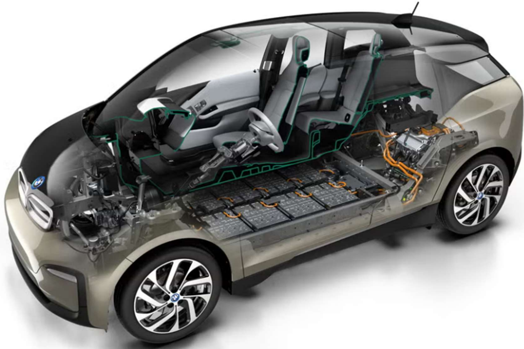
Figure 10. Battery Layout in Electric Vehicle
